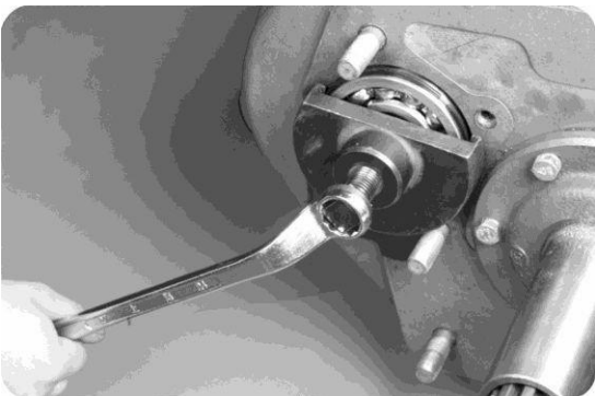
17, from the forward after knocking counter shaft, bearing retainer ring from the housing with at least 5 mm, bearing down counter shaft front with special tools.
