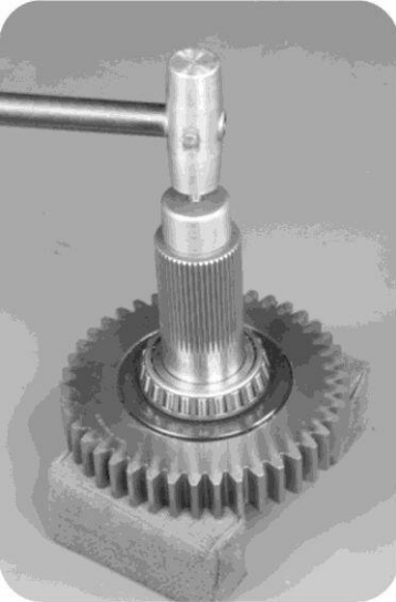
13, the knock on the output shaft and the bearing separation.
