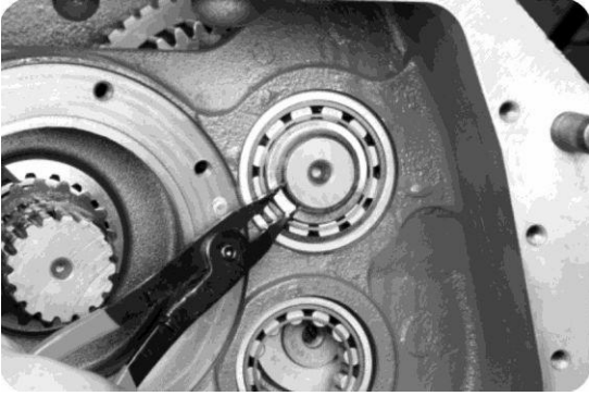
14, remove the main bearings on the counter shaft box rear stop ring.
