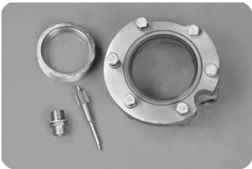
17, the output of the bearing cap bolts removed, remove the bearing cover, remove the speedometer and odometer joint, passive gear.
