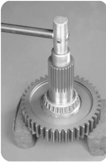
15, the output shaft assembly cushion, knock and remove the bearing.
