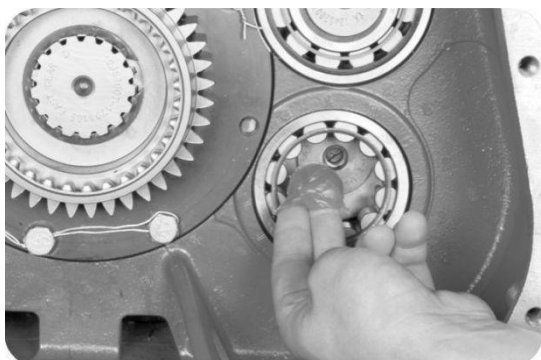
19, the grease evenly coated on the rear main box two counter shaft front bearing hole in (this step is very important).
