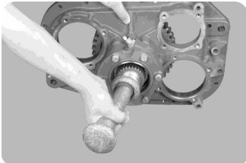
14, a backward output shaft, the bearing out from the hole.
