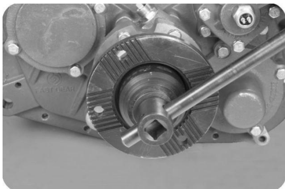
17, fasten the collar nut with a special sleeve.
