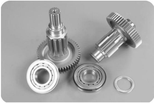
10, auxiliary box two counter shaft and bearing.
