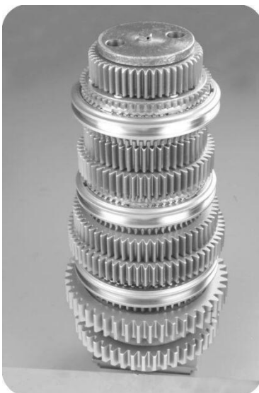
19, with press plate will a shaft gear fixed on the second shaft. (2) the main box counter shaft assembly assembly if auxiliary shaft of a gear needs to be replaced, counters haft gears of each stage in the press were under pressure, and will replace the gear in Figure 7-2 installation sequence of the press were pressed into the counter shaft. In two counter shaft
