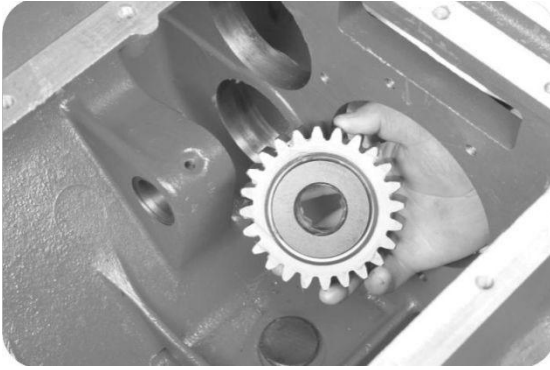
1, reverse gear wheel assembly, convex toward the front.
