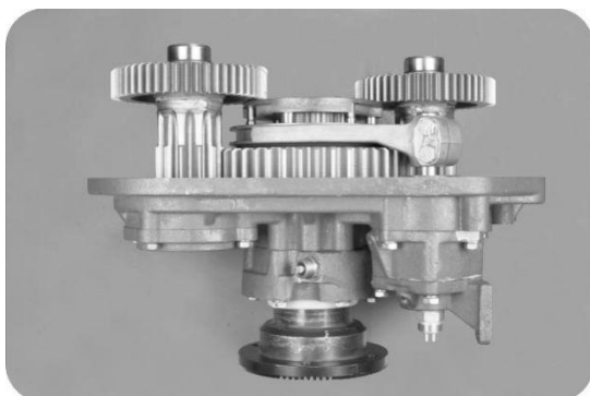
18, the sub box synchronization device in the low area.
