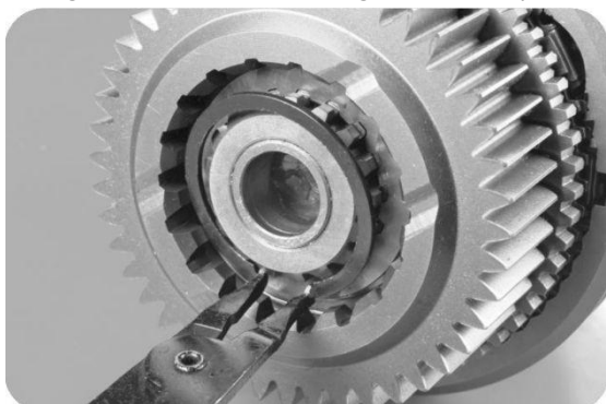
2, remove the stop ring in the inner hole of the shaft gear.
