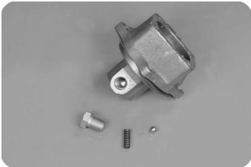
2, remove the bolt on the side of the cylinder shell, remove the positioning spring and steel ball.
