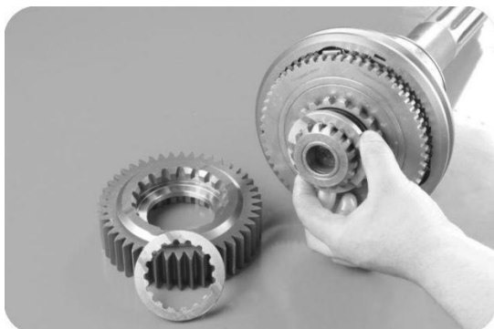
3, take off a shaft gear and its two side spline pad.
