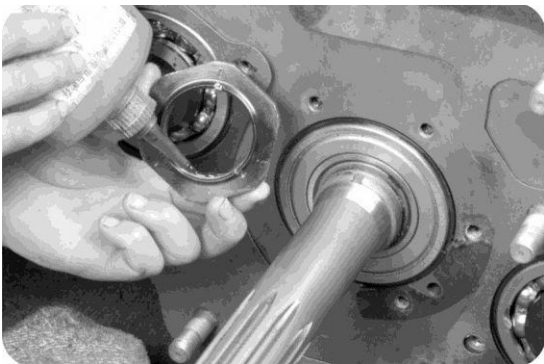
13, apply anaerobic adhesive on the screw nut thread.
