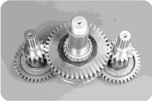
8, two pairs of teeth on the secondary gear reducer adjacent to the direction of the 180 pairs of teeth marks, as shown in figure.
