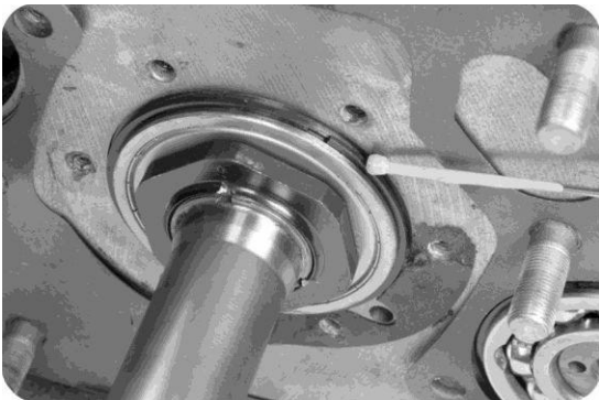
5, the assembly of a shaft bearing on the stop ring.
