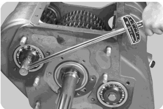
9, the upper right side of the rear shaft bearing assembly, and thrust ring for positioning.
