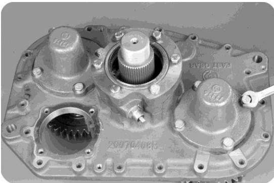
13, the assembly of the two end cap. Side gear shifting shaft cylinder parts decomposition is shown in figure 3-10.
