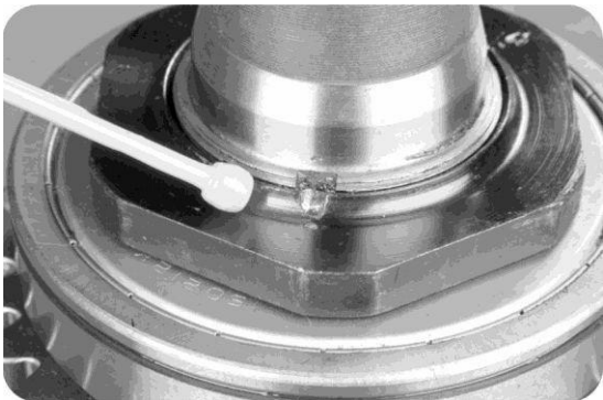
In 5, a shaft nut with anaerobic adhesive, tightening shaft nut and riveting die locking.
