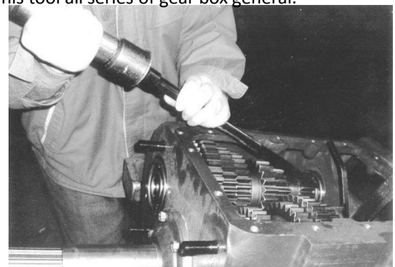
Figure 5B uses a fiber disassembling counter shaft bearing
