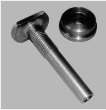
Figure 3A side box counter shaft front bearing puller
