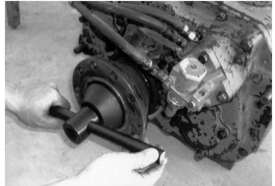
Figure 9b removable collar nuts with a special sleeve
