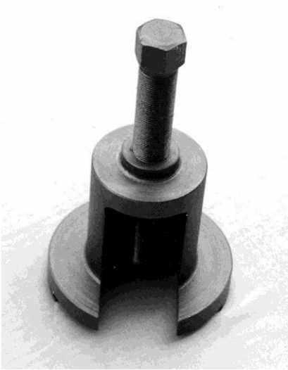
Figure 11a auxiliary box counter shaft bearing puller
