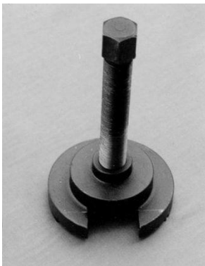
Figure 2A the main box counter shaft front bearing puller
