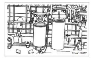
(b). Dismantle the fuel fine filter with a fuel filter wrench.
