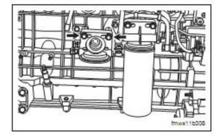
(b). Dismantle the fixing bolt of the oil-water separator seat.
