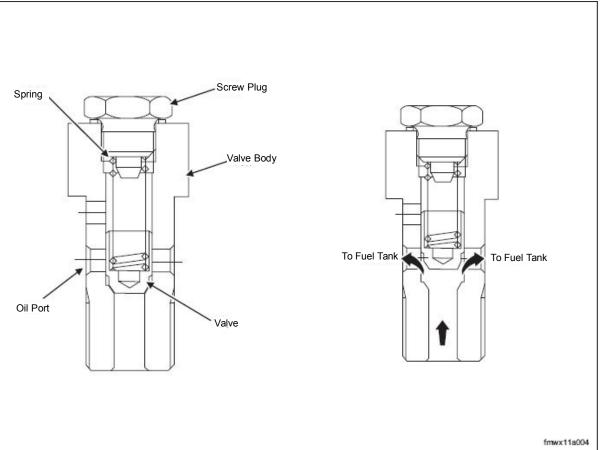
The low-pressure fuel feed side of the high-pressure fuel pump is connected with the fuel inlet of the fuel metering valve in parallel and is provided with a fuel return valve. The valve enables the low-pressure fuel path to keep a constant fuel feed pressure, and the fuel return pipeline of the high-pressure fuel pump is connected out of the fuel return valve.
