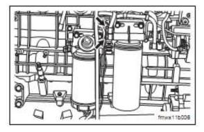
(c). Install the inlet and outlet pipes of the fuel fine filter.
