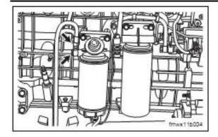
(b). Install the hinged bolts of the inlet and outlet pipes.
